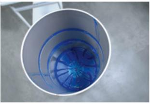
Emptying of drums to less than 1 % residue.\*
