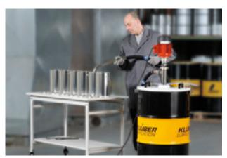
Filling of high-temperature lubricating grease.\*
