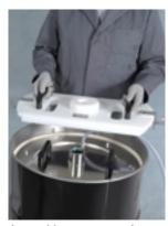
Assembly pump centring plate.\*
