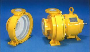
Process pump for corrosive media and heavy duty applications. Designed to international standards DIN 24256, ISO 2858. Pump casing lined with thermoplastic resins using ILS<sup>™</sup> technology. Provides excellent resistance to both high pressure and vacuum.
