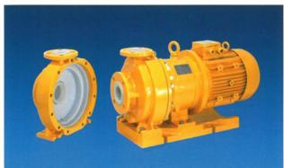
Process pump for corrosive media and heavy duty applications. Same properties as for the UTN-L, features an enclosed one piece impeller/magnet assembly. Reliable and simple, no pump/motor alignment required with close-coupled design.
