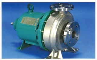
Heavy duty, metallic chemical process pump, designed to international standards DIN 24256, ISO 2858. Pressure rating up to PN40. Reliable and tireless with optimised radial bearing lubrication. Axial thrust is always under control with the 'on board' LSC<sup>™</sup> system, and very low NPSH requirements due to impeller manufacturing technology.
