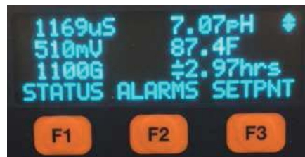
Figure 4A Screen if any alarm present
