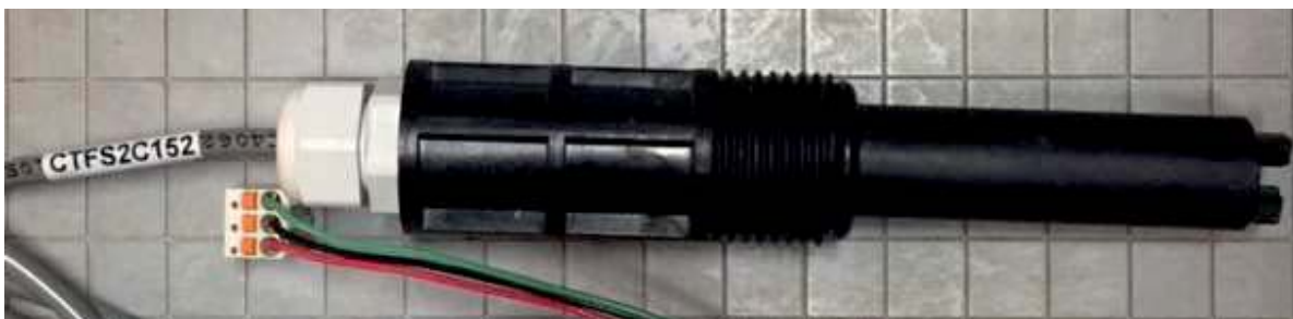
Figure 38 CTFS sensor (Conductivity/Temperature/Flowswitch/Serial)
