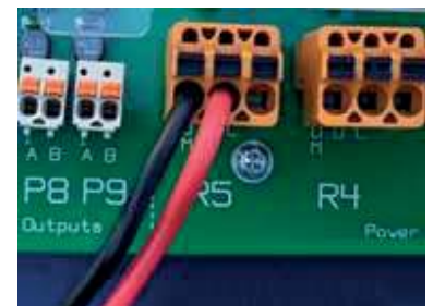
Figure 26 Using external power
