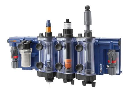
The BAMa modular sensor bypass assembly accommodates ProMinent sensors for water treatment. The assembly is simply installed in a bypass of the main process line. It is available in various variants, each perfectly designed for special water treatment applications – from drinking water, water for pool & wellness to industrial water.
