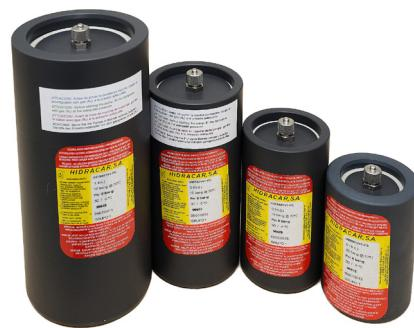
**Note:** Dampers are supplied uncharged & have to be filled according to the pressure in the system they will be installed in with either dry nitrogen or air. As a rule of thumb 70% of line pressure.
